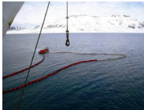
PyroBoom & GlobeBoom Being Readied for Tow Testing
